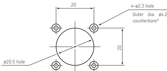
Note: 1) In case JC with a dust-proof rubber cover, the counterbore-work (\*part) is not necessary.
